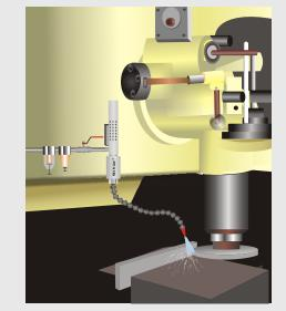
A Series of Model 57015FS Frigid-X<sup>™</sup> Tool Coolers are used to cool the slitting cutters in a continuously moving paper roll slitting machine.
