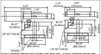
MINI SPOT COOLER WITH MUFFLER MINI SPOT COOLER
