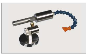
The Mini Spot Cooler utilizes a vortex tube to create one hot stream and one cold stream (see page 9). The cold air produced at the cold end is directed to the surface to be cooled using a flexible hose.
